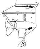
(2) Insert the oil tube nozzle into the lower oil plug hole, and fill with gear oil by squeezing the oil tube until oil flows out of the upper plug hole.
