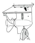
③ Install the upper oil plug, and then remove oil tube nozzle and install the lower oil plug.
