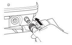
③ Feed fuel to the carburetor by squeezing the primer bulb until it is firm.
